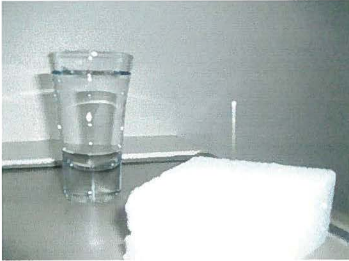
Image D: Proposed method for soaking probes utilizing a piece of Styrofoam
