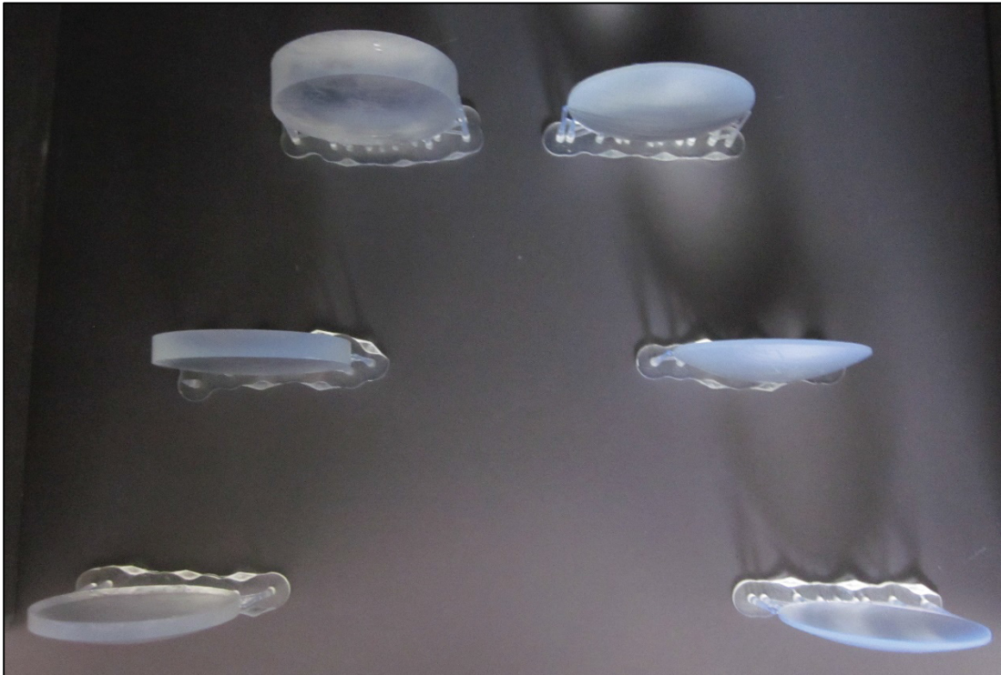
Figure 3: Unpolished printed lenses top view. Left to right: -2.00D, -5.00D, -10.00D, +2.00D, +5.00D, +10.00D.
