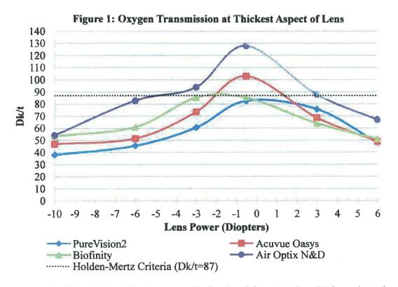
Air Optix Night & Day lenses maintained a Dk/t greater than 87 throughout the lenses in powers ranging from about -4.50D to +3.00D. Acuvue Oasys lenses in a narrow range of powers from roughly -2.00D to +1.50D that also remained above this threshold.
