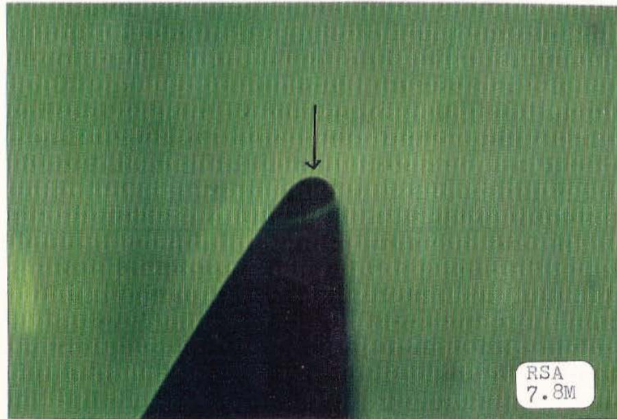
Figure 5: Edge profile of a lens with unacceptable forward apex (top). The bottom photograph shows this same lens after modification.
